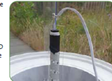
The light sensor is attached to the screw.
